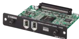
Optional FW16E Firewire Expansion Board
